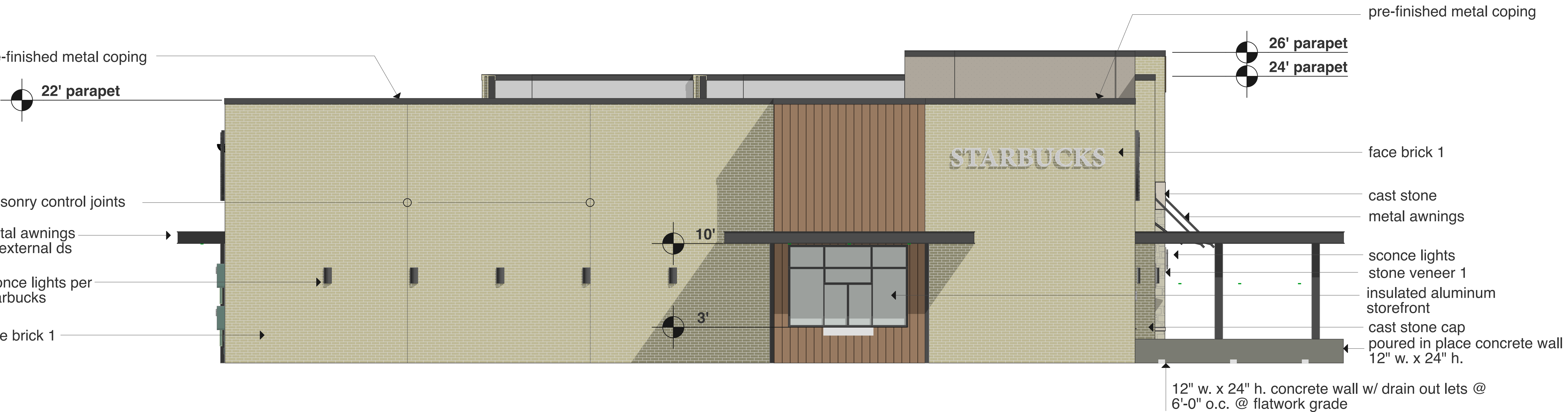
03 Left Side Elevation (South) SCALE: 1/4" = 1'-0"
