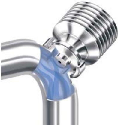
K-Patents Compact Process Refractometer PR-23-GC is designed for the general industry small pipeline and bypass line applications. The PR-23-GC sensor is easy to install in the process either directly in a pipe elbow by a Sandvik coupling connection or in a straight pipe via a Wafer flow cell or a Pipe flow cell.
