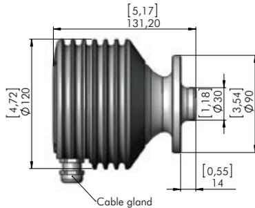
Sensor PR-23-GC with WFC Wafer flow cell (1 inch)
