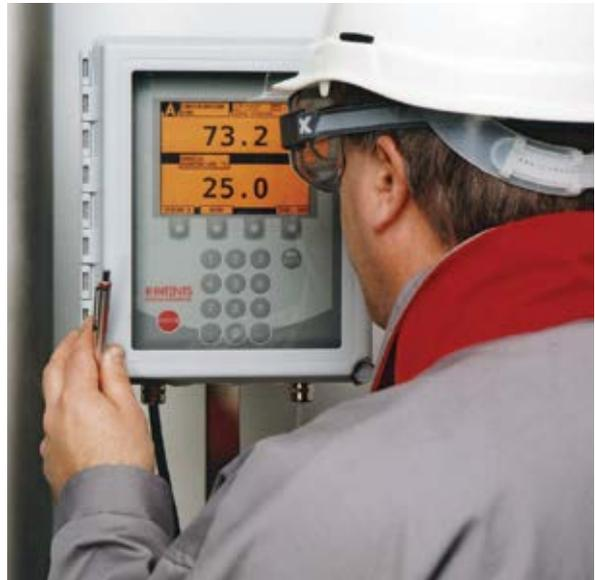
COMPACT PROCESS REFRACTOMETER PR-23-GC
