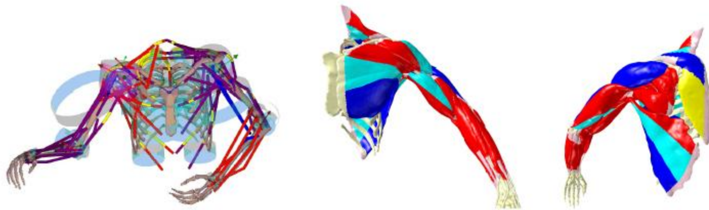
Fig. 4. The leftmost figure shows the piecewise linear muscle models with wrapping surfaces to model muscle contact in inverse dynamics calculations. Larger muscles have multiple contractile regions with individual activations and these must be embedded in the tetrahedron meshes for simulation (rightmost figures).
