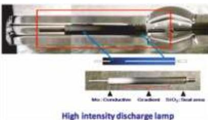
Fig .13 High Intensity Discharge Lamp
