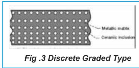
**Fig .3 Discrete Graded Type**
