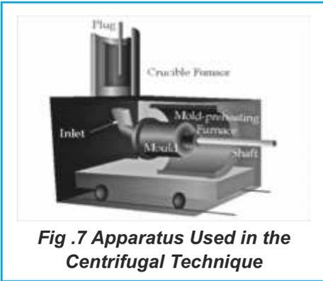
**Fig .7 Apparatus Used in the Centrifugal Technique**
