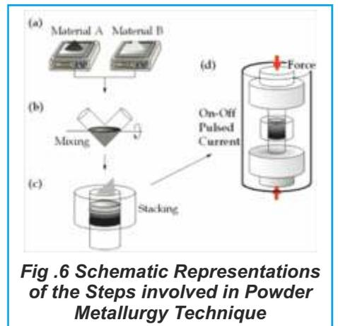
**Fig .6 Schematic Representations of the Steps involved in Powder Metallurgy Technique**
