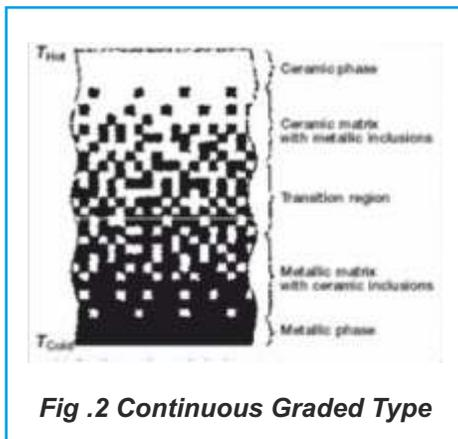
**Fig .2 Continuous Graded Type**
