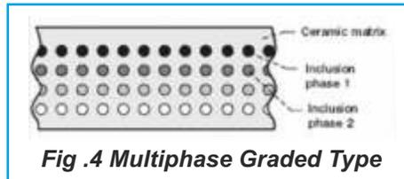
**Fig .4 Multiphase Graded Type**
