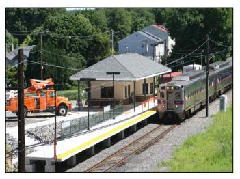
New Station Building and High Level Platform This project provided for the reconstruction of station facilities at Cheltenham Station on the R8 Fox Chase Line. Improvements included a new high-level pre-cast platform; a station building with ticket office, waiting area, and restroom facilities; enhanced lighting; and signage. The new station is fully ADA accessible. This project was completed August 2007.
