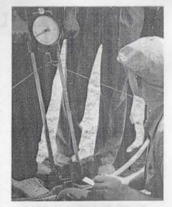
Shown above is the bow weighing machine used by the National Archery Association to weigh Flight bows in various classes. A bow is placed in the machine, the string is drawn to the desired draw length as shown by a pointer and the pounds pull is registered on the scales above.
