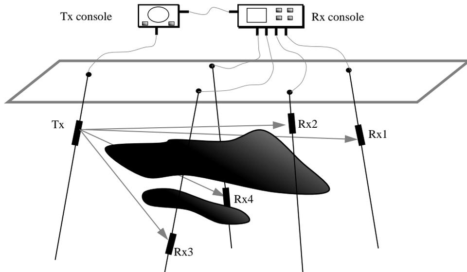
Figure 3. Schematic diagram of a 3D cross-hole EM exploration system with a transmitter (Tx) in one borehole and multiple receivers (Rx) in multiple boreholes.
