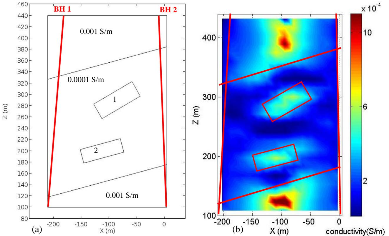
Figure 2. (a) The borehole plane section view of the synthetic 3D model with conductor 1 (perfect conductor) and conductor 2 (with a conductivity of 0.01 S/m) in a layered background. The strike length of the two conductors is 60 m and both are symmetric across the borehole plane ( $y = 0$ ). (b) Inverted conductivity model.
