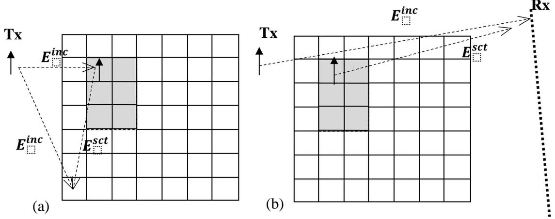
Figure 1. Discretization of a borehole plane for inversion. (a) Scattered field from a cell to another cell; (b) scattered field from a cell to a receiver location.
