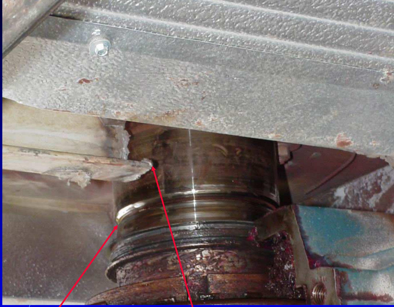
Figure 6. Groove Worn In Fan Shaft Caused by Continuous Contact With Rubber Air Seal.
