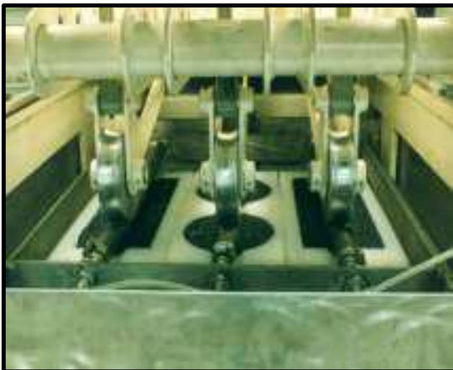
APA Rut Testing (Beam/Cylindrical Samples)
