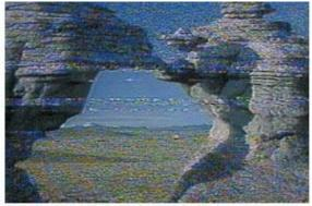
Interference caused by a thermostat
