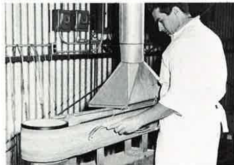
Sawing out the handle of the PRESENTATION—one of the many precise operations in making this beautiful bow.
