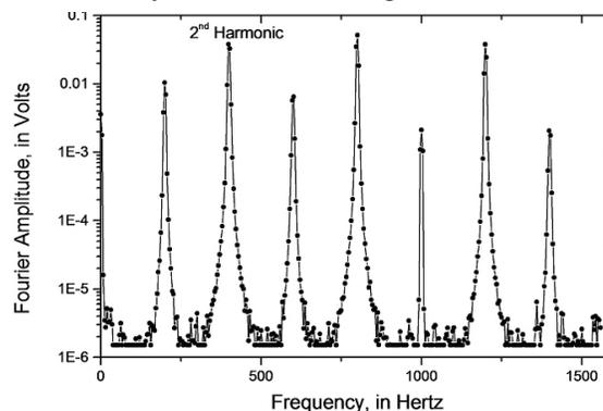
Figure 5: Output signal of the Fluxgate Magnetometer in a 3 mT magnetic field.
