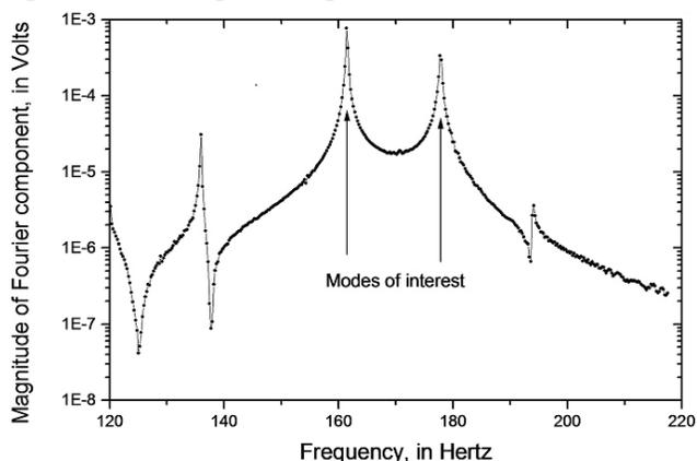
Figure 2: Coupled Oscillator Chirp Signal
