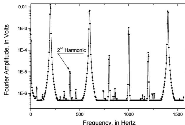
Figure 4: Output signal of the Fluxgate Magnetometer driver at 200 Hz in a zero magnetic field. The various harmonics are clearly visible at 400, 600 and 800 Hz.
