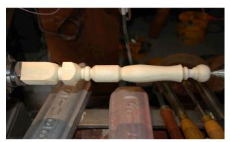
must be made from larger diameter to smaller diameter. This is necessary to make the cut as smooth as it can be made. The reason the cut is as smooth as it can be is because the fibers in the wood are being cut in such a way that the underlying fiber is supporting the fiber that is being cut. If you try to cut the other way the tool will lift the grain and it will chip out very badly and leave a rough surface.
