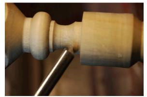
the tool and scoop out the wood. Work a little on one side and a little on the other till you have a finished cove that is both wide enough and deep enough.
