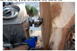
the tailstock. You can now start the lathe without turning the speed all the way down because it is already balanced.
