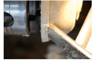
What about the speed of the lathe? The lathe should not be turned fast enough to make it shake, but should be turned fast enough so that small differences in the "hardness" of the wood do not set up vibrations in the cut. You have had occasions where you feel a rough surface on the wood that
