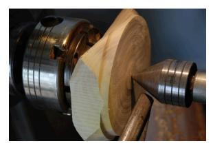
I will continue the line of cut till the blank is round and has straight sides.
