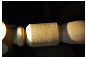
you just cut. When you shut the lathe down you see a spiral pattern on the surface of the wood, that is because there are differences in hardness of the wood (late wood, early wood) and the speed of the wood past the tool allows the tool to "dip" into the softer wood then "bounce" out when the harder wood comes by this leaves a low spot and a high spot. When these come around again it amplifies the dip and bump and creates a new one a little
