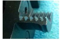
easier to make the spigot that fits these jaws. When you make the spigot to grip on the outside remember to make room for the tooth, if you don't it will try to bite the spigot off of the bottom of the bowl, and it will be successful more often than you would like it to be. The spigot should never touch the inside bottom of the jaws, always make the spigot so that the wood registers against the outside top of the jaws.
