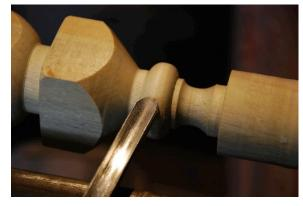
What happens if you don't ABC? A design change opportunity will be made available to you! If you stick the cutting edge into the rotating wood before you anchor the tool on the tool rest, the wood will anchor the tool for you! If you lift the handle too much and create a situation where the 2 points of contact are the tool rest and
