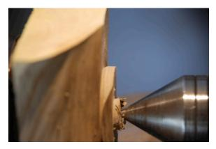
I then mounted the blank in the jaws by the spigot with pressure from the tailstock to help set the jaws while tightening and providing a little extra safety while knocking off the corners.
