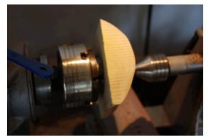
and held in place with the tailstock and rotated and adjusted to center.
