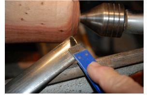
restore the edge many times before you need to regrind the skew. When the little flat spot, or mini bevel, is 1/16'' to 1/8'' you should consider regrinding.
