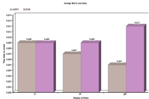
Fig. 12. Average end to end delay Comparison for AODV and DSR
