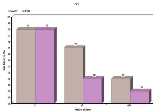
Fig. 13. Packet Delivery Ratio Comparison for AODV and DSR
