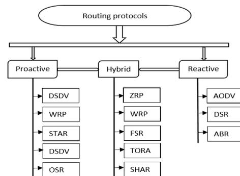
Fig. 1. Classification of Routing Protocols
