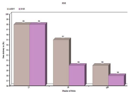
Fig. 13. Packet Delivery Ratio Comparison for AODV and DSR
