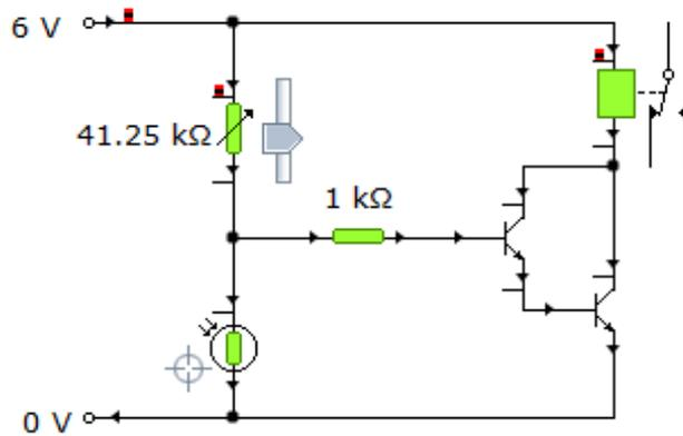
7 (c)(i) Add a component to prevent back e.m.f. from the relay coil causing damage to the transistors. [2 marks]
