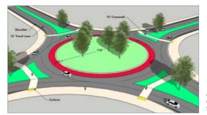
*Figure 53: A typical Roundabout* layout suggests reserving a servitude width of at least 180!
