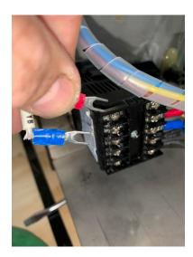
3.BEFORE INSTALLING NEW PROBE JUST HOOK IT UP TO CONTROLLER AND THEN TURN UNIT ON TO SEE IF IT READS AMBIENT TEMPERATURE. IF IT SEEMS TO WORK GO AHEAD AND TURN POWER OFF AND PROCEED TO REMOVE OLD PROBE AND REPLCE WITH NEW PROBE.
