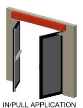
LH Operator (counter-clockwise swinging doors)
