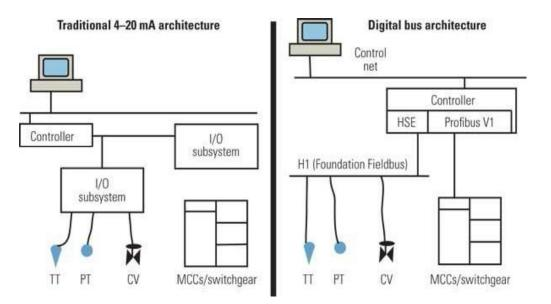
**Old and new.** This diagram compares a traditional analog architecture with the new digital bus architecture for power plant controls. Source: Fluor
