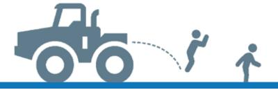
Hop or shuffle away from an energized line until you are 10 meters (33 feet) away
