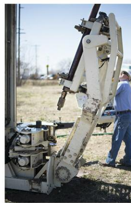
Running sonic weighted wireline with SDT45 tooling. (above) Modular weight assembly, with the overshot 'spear' visible inside the weight head prior to being lowered downhole. The modular weight assembly consists of two, 150-lb. weight segments coupled together and a threaded head and overshot spear.
