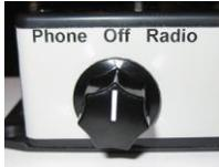
**Off** – Both phone and Ham radio will be disabled. Switch your interface to “Off” when getting ready to race to ensure you are not disturbed on stage.
