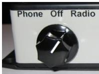
**Radio** – Listen to your Ham or Commercial radio. Monitor the Rally Net or communicate with your service crew while in transit. The PTT button is required to transmit. While the PTT button is depressed, both the Driver and Co-Driver can transmit over the radio.
