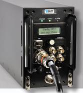
The new SkymasterTX (SKTX) is a lightweight, full-featured digital COFDM video downlink transmitter built to address the unique requirements of aircraft downlink operation. The chassis design features either horizontal or vertical ARINC mounting. All of the connections and controls have been located on one side of the unit. This allows the SkymasterTX to be removed from one aircraft and installed in another with ease.
