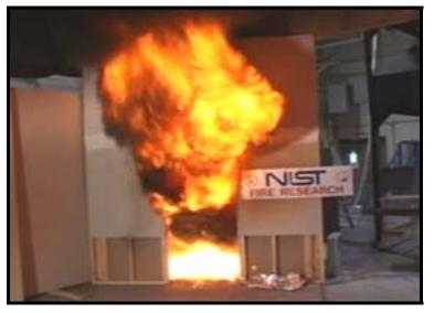
Figure 3 – Flashover and subsequent Backdraft
