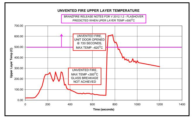
Figure 9 – Upper Layer temperature for the Unvented Fire
