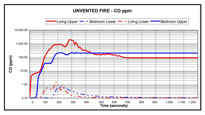
Figure C4 <u>Upper Layer</u> Carbon Monoxide Levels (CO) for unvented fire simulations This graph is provided for Fire Engineers' interest only.
