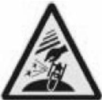
Note: when press the tire, the opened clamp cylinder may injure the hand of the operator. Remember, do not touch the side wall of the tire.
