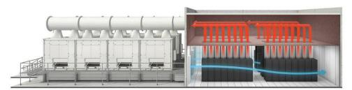
The methods above contain an entire aisle; however, in cases of scattered high density racks, it may make sense to contain individual racks using a duct. With this method, a duct is mounted to the back of the rack to contain the hot exhaust air, and then is ducted into the
