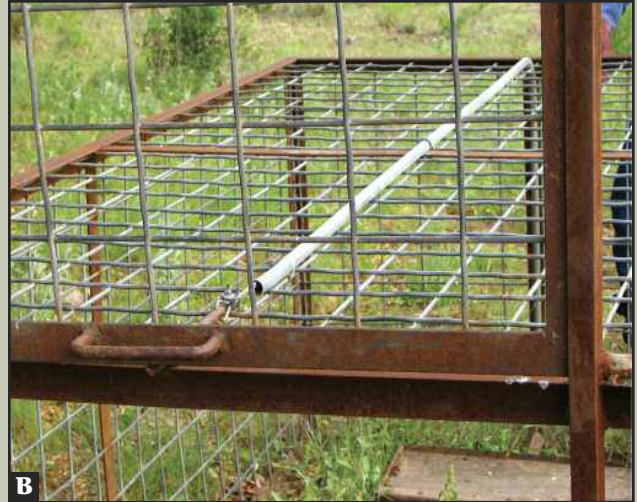
Many drop gates use a pin or similar object attached to a cable to hold the trap gate open (A). The cable can be slid through a conduit to the back of the trap, where it is attached to a trigger system (B). Trigger systems vary in design. (Source: Terry Gallagher)
