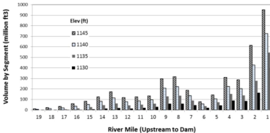
Figure 5. Reservoir volume by mile segment at different water elevations.
