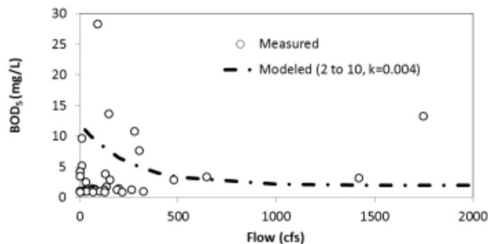
Figure 9. Measured biochemical oxygen demand (BOD<sub>5</sub>) in the reservoir and predictive relationships between flow and BOD<sub>5</sub> used in the model. Modeled inflow BOD ranges from 10 mg/l to 2 mg/l with a first order reduction as flow increases.
