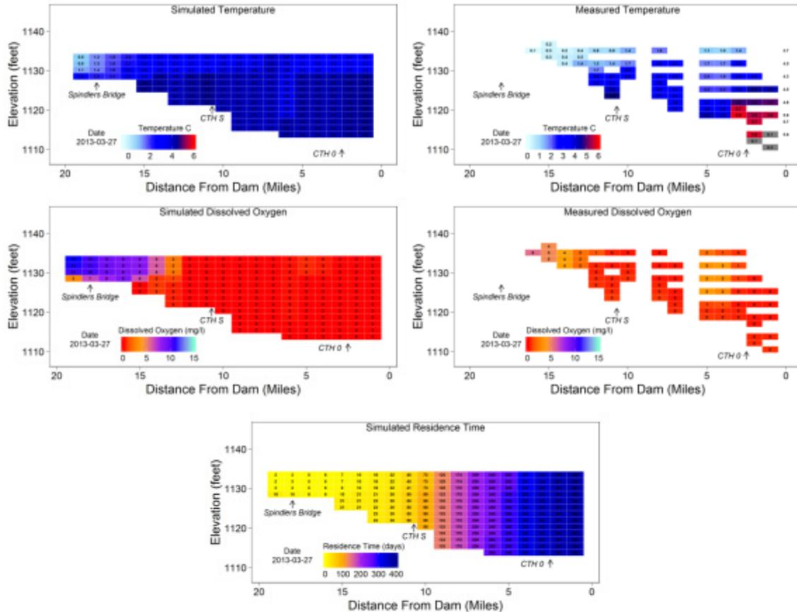
**Figure 24. Simulated and measured temperature (upper), dissolved oxygen (middle) and residence time (lower) in the Big Eau Pleine Reservoir on March 27, 2013, more than 120 days after ice formation.**
