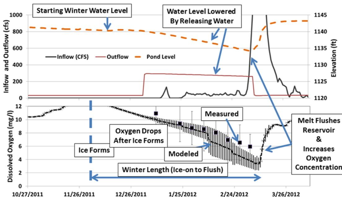
Figure 2. Comparison of water level operation (above) and dissolved oxygen concentrations (below) during a typical winter in the Big Eau Pleine Reservoir
