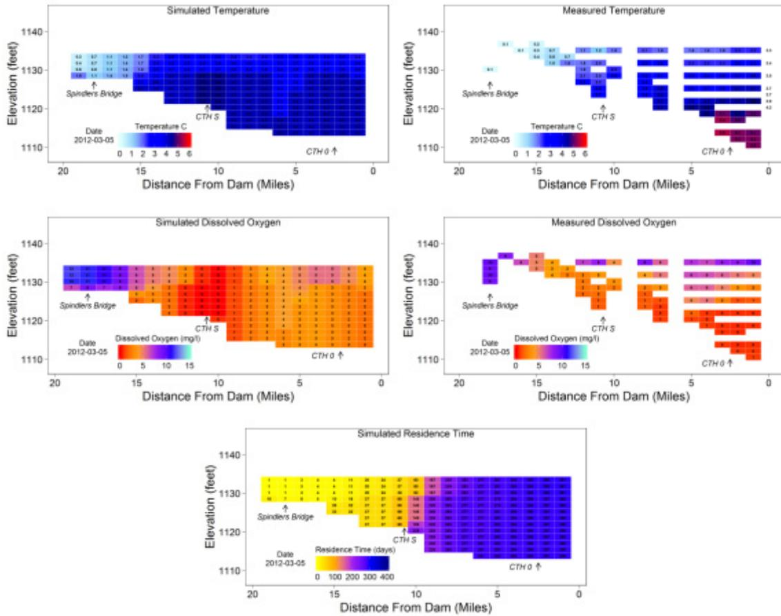
Figure 15. Results of model simulation and measured results for dissolved oxygen, temperature and residence time from early March 2012 approximately ninety days after ice formation.
