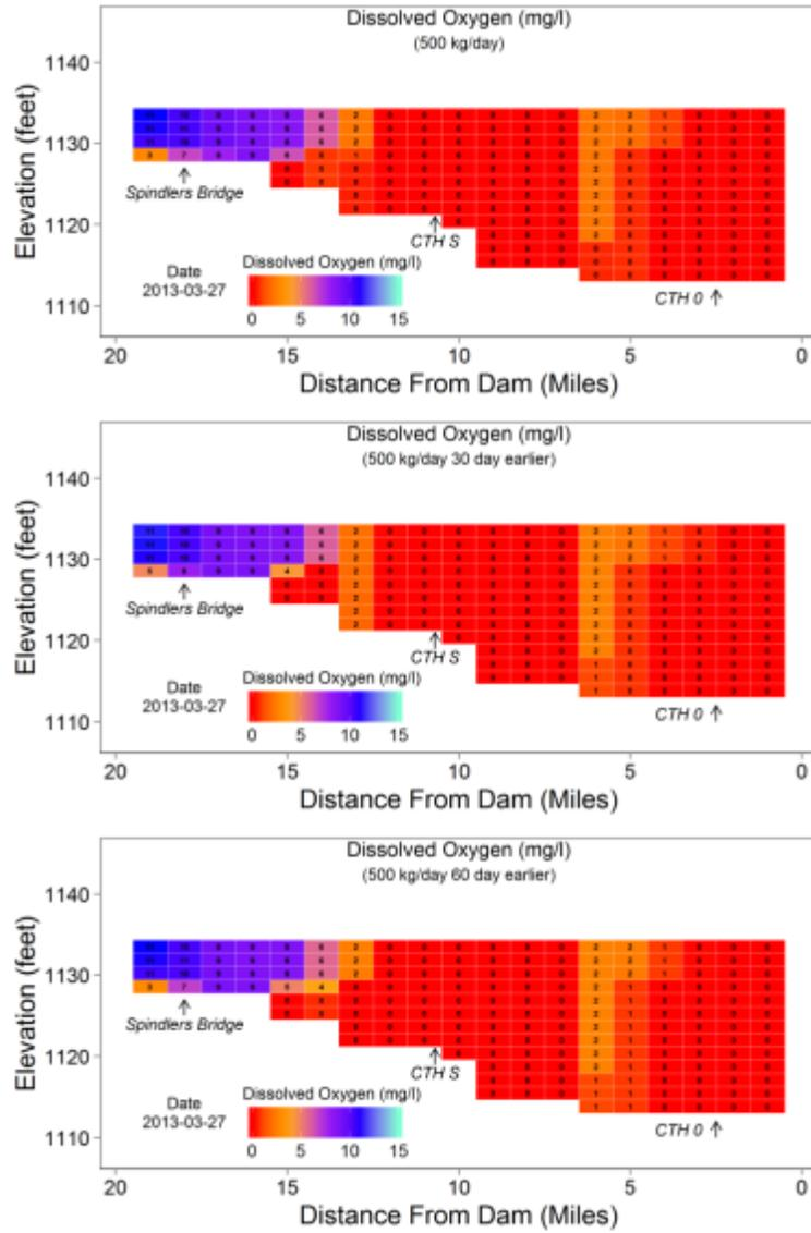
Figure 37. Comparison of dissolved oxygen profiles in the Big Eau Pleine Reservoir for March 27, 2013 comparing earlier start of the aerator. Upper profile is simulated 500 kg/day starting on February 13, second is 500 kg/day starting 30 days earlier, third is 500 kg/day starting 60 day early.
