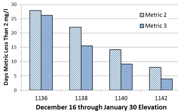
Figure 32. Comparison of days that Metric 2 and Metric 3 were under 2 mg/l in simulations that started on December 16 but remained at that elevation through January 30 before drawing down to 1135 by March 30.
