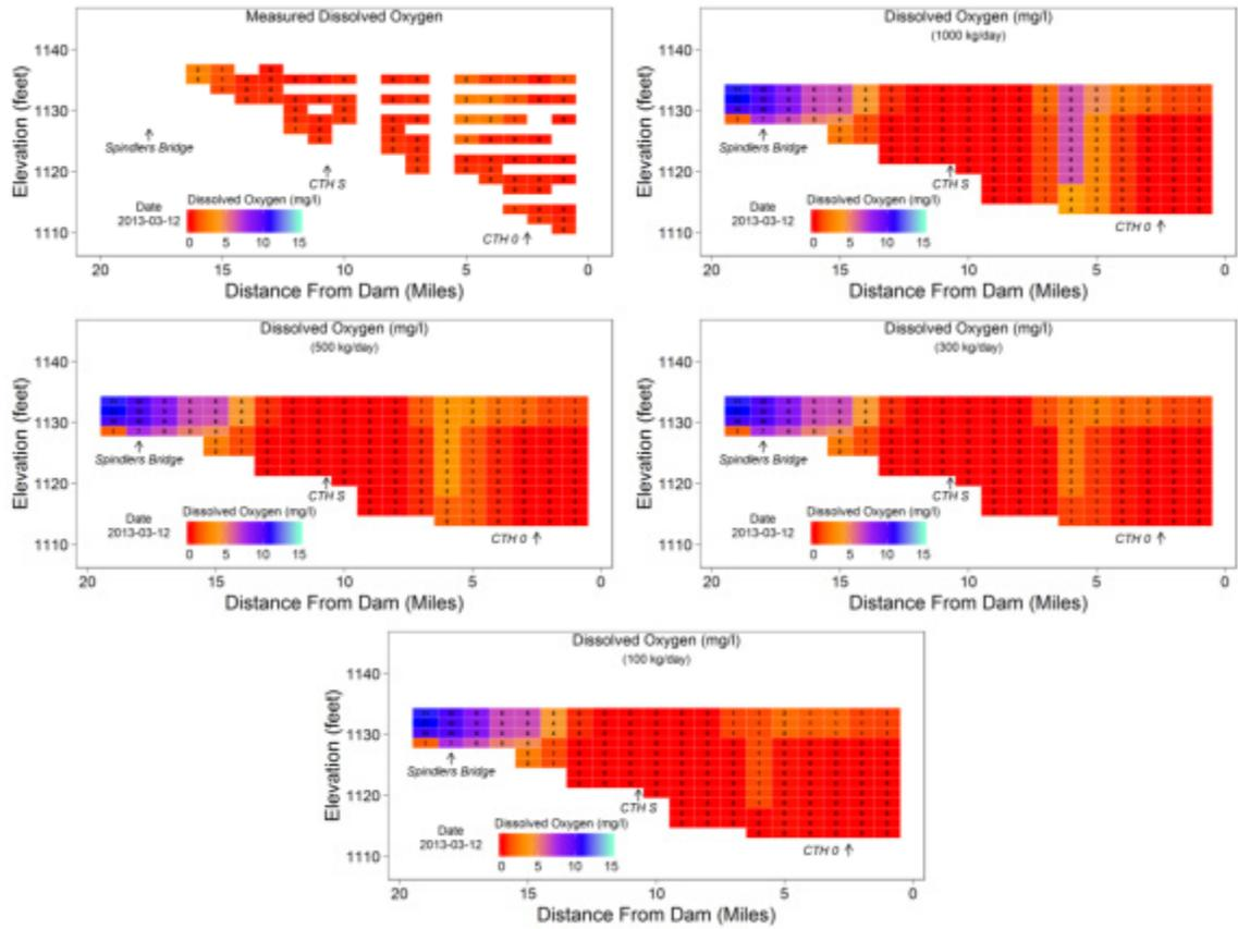
Figure 34. Comparison of dissolved oxygen profiles in the Big Eau Pleine Reservoir for March 12, 2013, four weeks after the start of aeration. Upper profile is measured followed by simulations of 1000, 500, 300 and 100 kg/day of oxygen.
