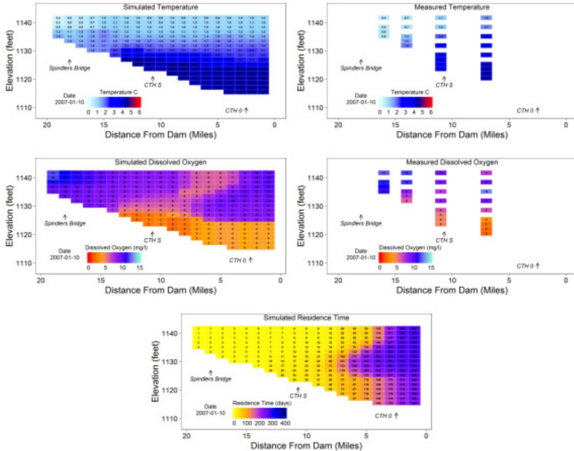
**Figure 17. Simulated and measured temperature (upper), dissolved oxygen (middle) and residence time (lower) in the Big Eau Pleine Reservoir on January 10, 2007, approximately five weeks after ice formation.**
