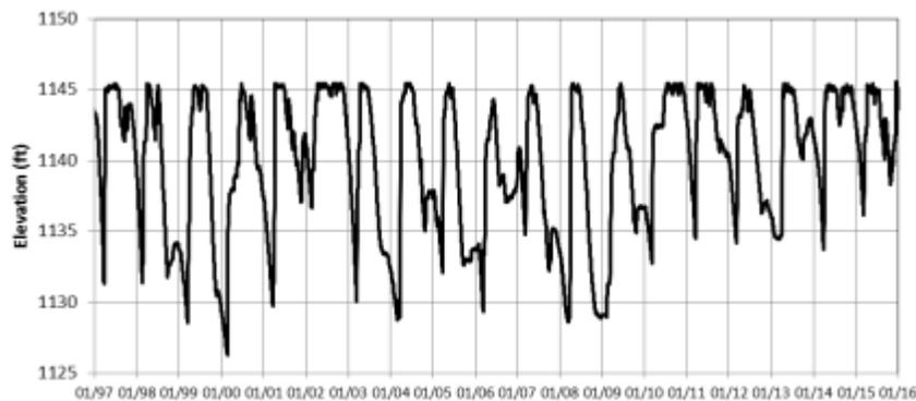
Figure 27. Reservoir elevations from January 1997 through 2015 (WVIC).
