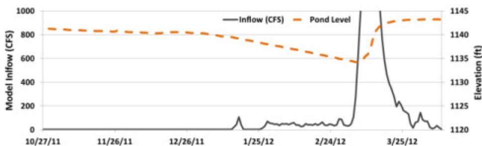
**Figure 12. Variation in inflow (solid line) and reservoir elevation (dashed line) during the 2012 winter.**
