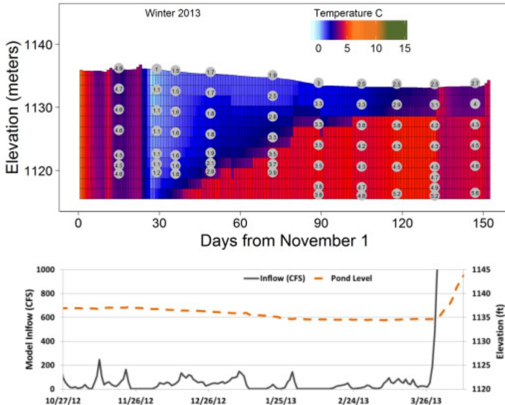
**Figure 20.** Upper figure shows the measured and modeled temperature during the 2013 winter. Lower figure shows the inflow (solid line) and reservoir elevation (dashed line).
