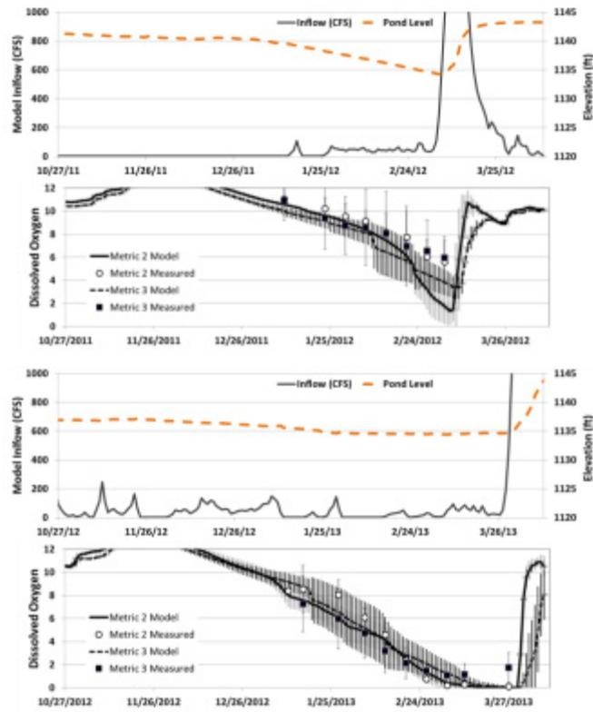
Figure 26 (continued). Comparison of the reservoir inflow and reservoir elevation (left) and the model metric dissolved oxygen concentrations tracked through each winter. Measured metric values shown as mean plus and minus one standard deviation for the measurements within the metric on that day. Range around the model metric values is the standard deviation within metric model segments on that day.
