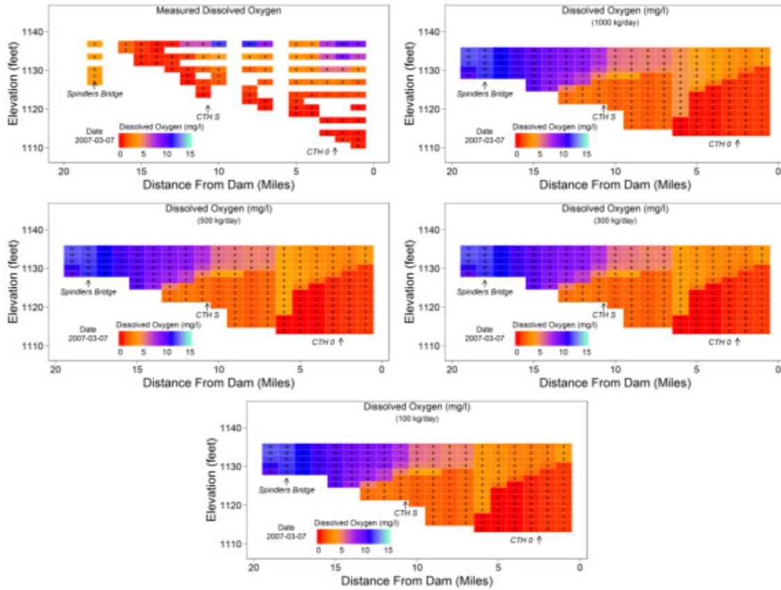
**Figure 36. Comparison of dissolved oxygen profiles in the Big Eau Pleine Reservoir for March 7, 2007, two weeks after starting aeration. Upper profile is measured followed by simulations of 1000, 500, 300 and 100 kg/day of oxygen.**
