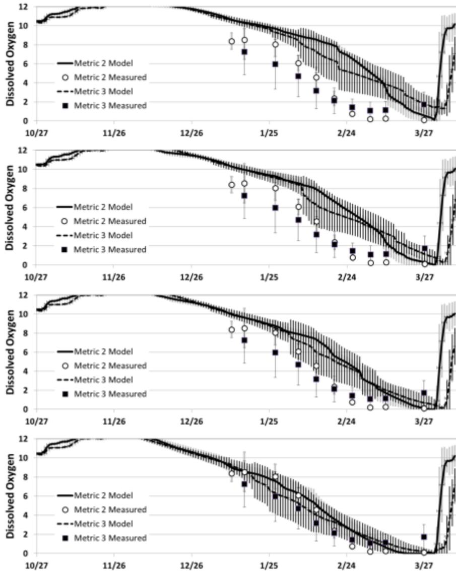
**Figure 30. Comparison of Metric 2 and Metric 3 over time simulated with progressively lower starting elevation on December 16 (top: 1142, 2<sup>nd</sup>: 1140; 3<sup>rd</sup>: 1138; bottom: 1136) with all simulations ending at 1135 feet on March 30. Measured results from 2013 shown for comparison with these synthetic simulations.**
