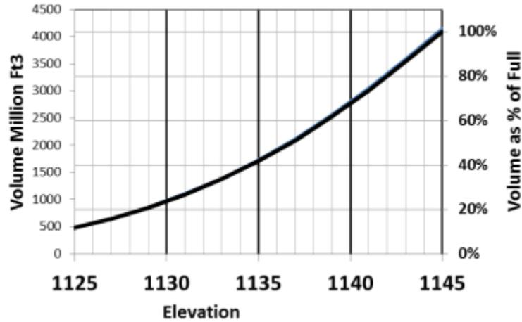
Figure 4. Relationship between reservoir water elevation and both the volume (left) and percentage of full reservoir volume (right).
