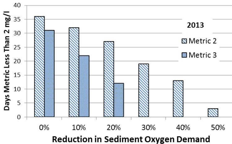
**Figure 41. Comparison of the number of days that Metric 2 (upstream of the aerator) and Metric 3 (downstream of the aerator) have on average dissolved oxygen concentration less than 2 mg/l in 2013 with changes in SOD. SOD reduction shown as a percentage reduction from the calibrated values.**
