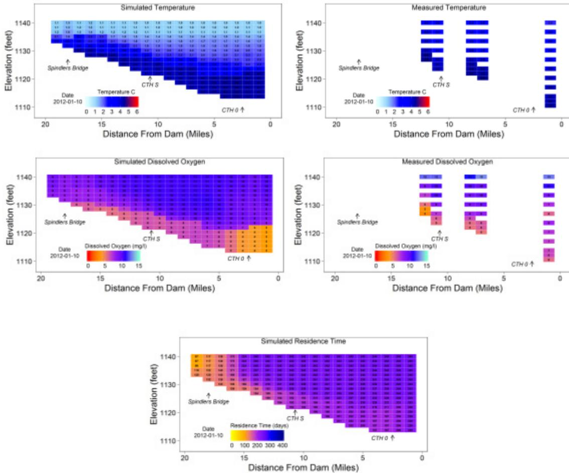
**Figure 13. Results of model simulation and measured results for dissolved oxygen, temperature and residence time from early January 2012 approximately thirty days after ice formation.**
