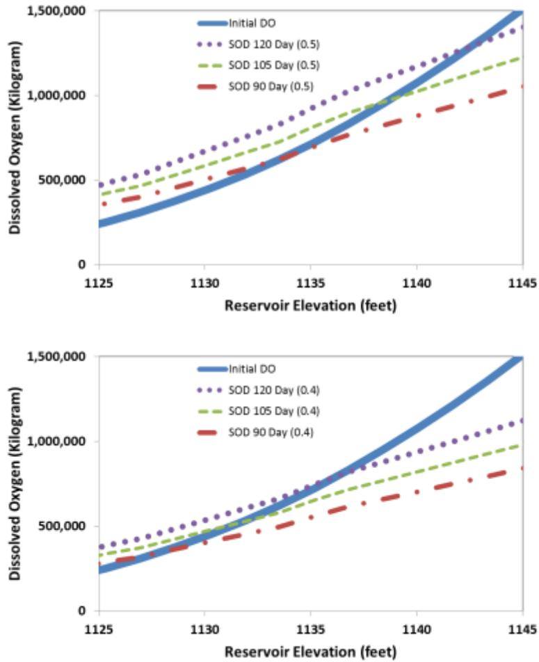
Figure 39. Comparison of the quantity of oxygen in the reservoir at the onset of freezing based on an initial concentration of 13 mg/l with the quantity of oxygen consumed at a sediment oxygen demand of 0.5 g/m<sup>2</sup>-day (upper) and 0.4 g/m<sup>2</sup>-day (lower). The sediment oxygen demand calculated for 90, 105 and 120 days after ice-on.
