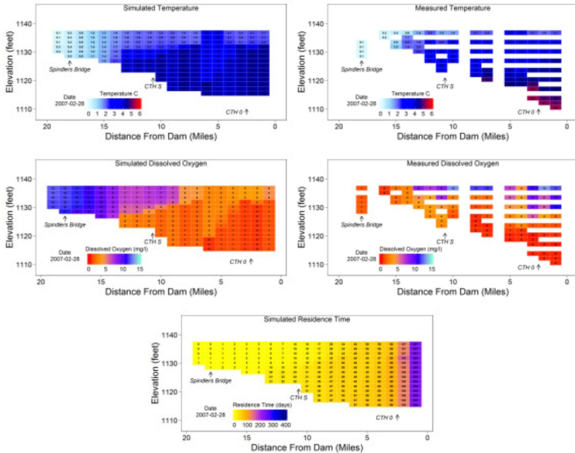
**Figure 18. Simulated and measured temperature (upper), dissolved oxygen (middle) and residence time (lower) in the Big Eau Pleine Reservoir on February 28, 2007, approximately eleven weeks after ice formation.**
