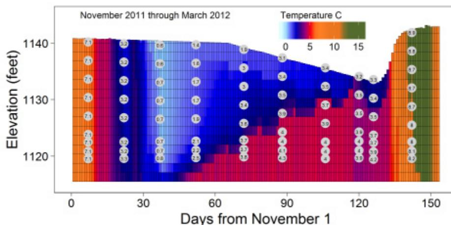
Figure 11. Measured (in circles) and modeled (color) temperature near the dam from November 2011 through March 2012.
