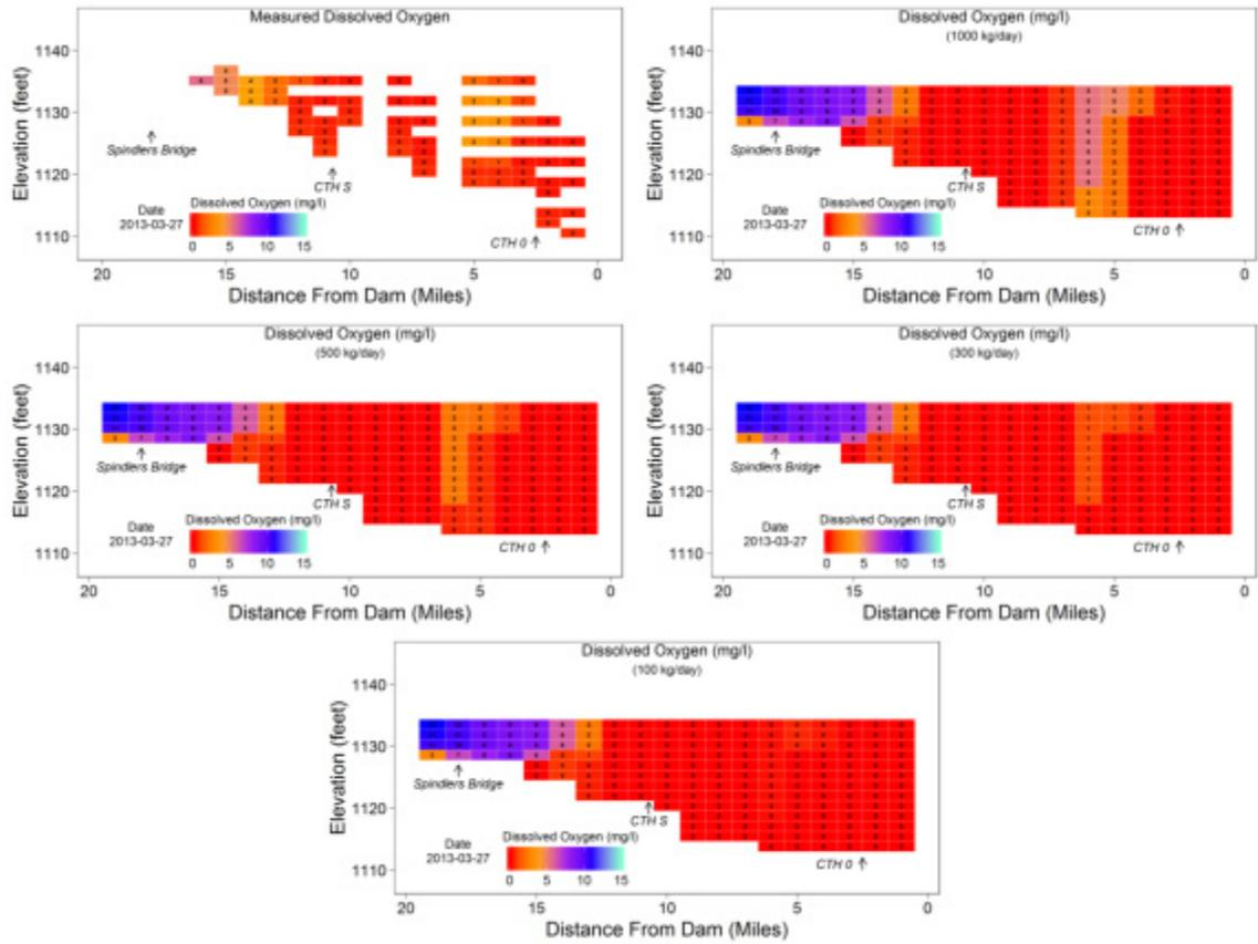
Figure 35. Comparison of dissolved oxygen profiles in the Big Eau Pleine Reservoir for March 27, 2013, six weeks after the start of aeration. Upper profile is measured followed by simulations of 1000, 500, 300 and 100 kg/day of oxygen.
