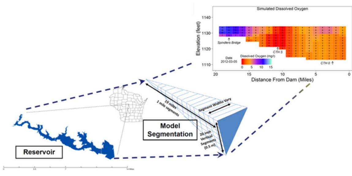
**Figure 1. Schematic illustration of how the Big Eau Pleine Dissolved Oxygen Model simulates the shape of the reservoir and calculates a dissolved oxygen concentration in the reservoir profile**
