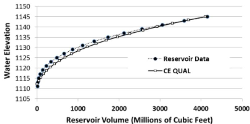
Figure 3. Volume/elevation relationship in the Big Eau Pleine Reservoir. Reservoir data provided by WVIC and the CE-QUAL data from bathymetry used in the model
