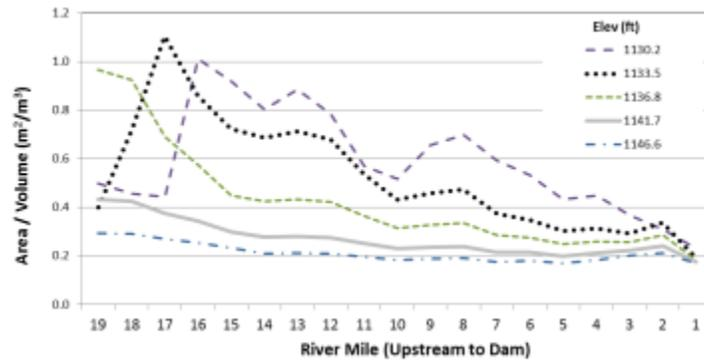
Figure 8. Changing ratio of sediment area to water volume at different locations in the reservoir at different water elevations.
