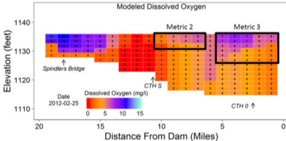
Figure 10. Reservoir cross section showing model results as dissolved oxygen concentration in each layer in each segment. Concentrations within the area for Metric 2 and Metric 3 were averaged for each day.
