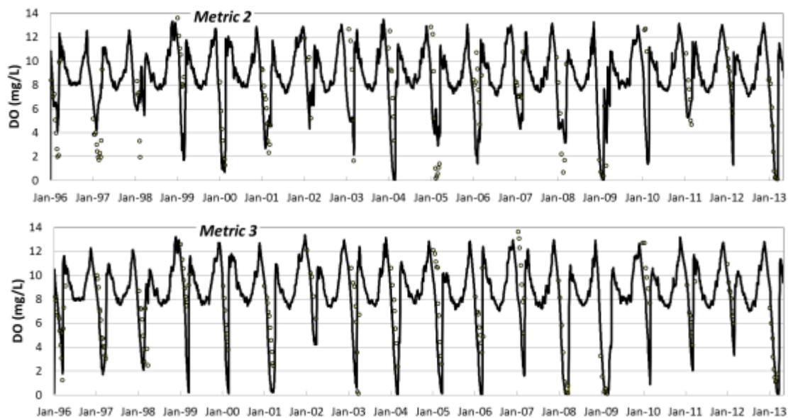
Figure 25. Daily average dissolved oxygen concentration measured within the Metric 2 (upper) and Metric 3 (lower) areas shown as symbols and the simulated for each day as lines.
