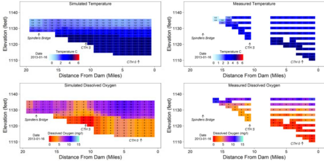
Figure 21. Simulated and measured temperature (upper), dissolved oxygen (middle) and residence time (lower) in the Big Eau Pleine Reservoir on January 16, 2013, approximately seven weeks after ice formation.
