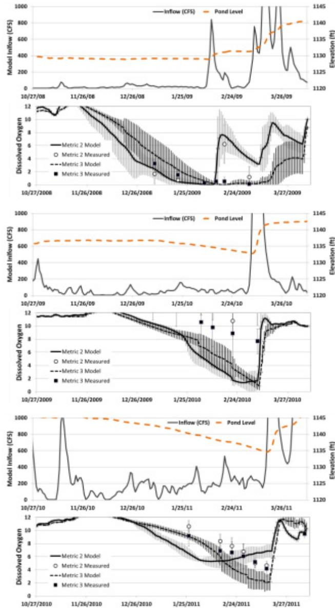
Figure 26 (continued). Comparison of the reservoir inflow and reservoir elevation (left) and the model metric dissolved oxygen concentrations tracked through each winter. Measured metric values shown as mean plus and minus one standard deviation for the measurements within the metric on that day. Range around the model metric values is the standard deviation within metric model segments on that day.
