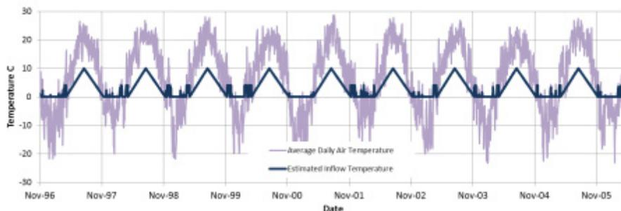
Figure 7. Comparison of the estimated inflow temperature for water entering the Big Eau Pleine Reservoir compared to the average daily air temperature. Inflow temperatures were linearly interpolated during the summer and matched to the maximum of air temperature or 0.1 degree C during the early winter.
