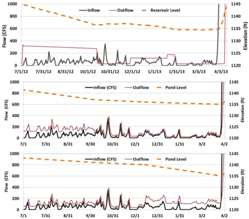
Figure 28. Example actual 2013 winter conditions (upper) followed by conditions used in the synthetic simulation of starting (12/16) and ending (3/29) elevations of 1136 to 1135 (middle) and 1140 to 1135 (lower). Pond level is the elevation of the water in the reservoir.
