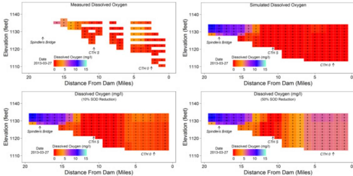
**Figure 40. Simulation results for March 27, 2013 with variations in the sediment oxygen demand (SOD). Upper left figure shows the measured profiles, upper right the model results with the calibrated SOD values, the lower left figure assumes a 10% reduction in SOD across the reservoir, and the lower right figure shows simulation with a 50% reduction in the SOD across the reservoir.**
