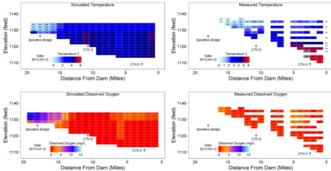
**Figure 23. Simulated and measured temperature (upper), dissolved oxygen (middle) and residence time (lower) in the Big Eau Pleine Reservoir on March 12, 2013, more than 100 days after ice formation.**
