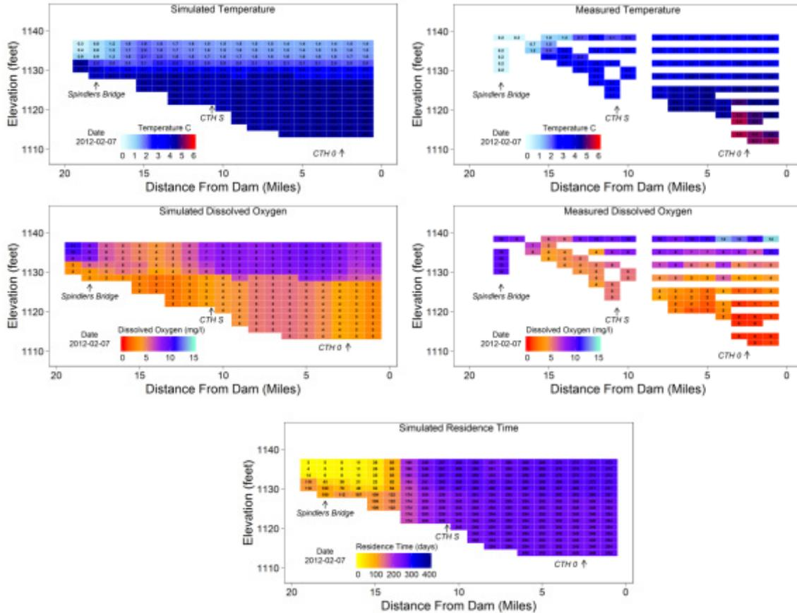
**Figure 14. Results of model simulation and measured results for dissolved oxygen, temperature and residence time from early February 2012 approximately sixty days after ice formation.**
