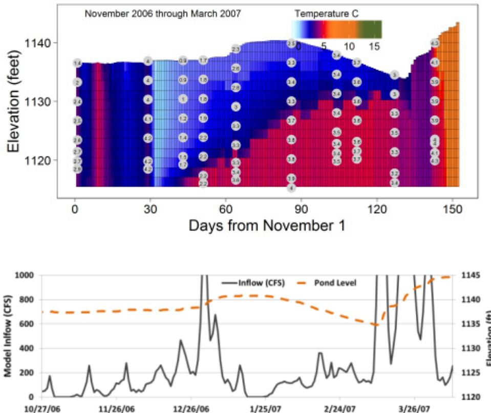
**Figure 16. Upper figure shows the measured temperature profiles (circles) and simulated temperature pattern (colors). Lower figure shows the variation in inflow (solid line) and reservoir elevation (dashed line) in the 2007 winter.**
