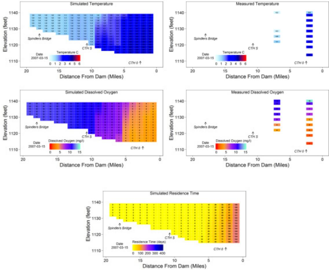
Figure 19. Simulated and measured temperature (upper), dissolved oxygen (middle) and residence time (lower) in the Big Eau Pleine Reservoir on March 15, 2007, approximately thirteen weeks after ice formation.
