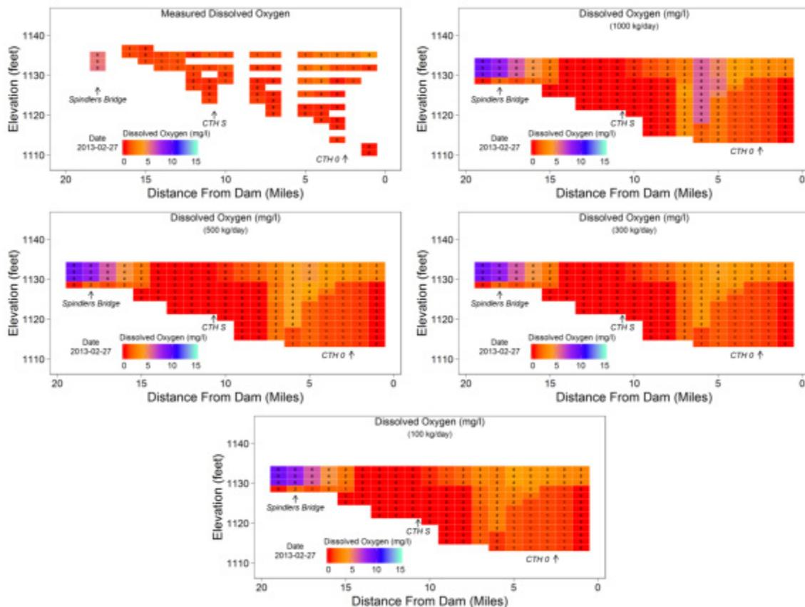
**Figure 33. Comparison of dissolved oxygen profiles in the Big Eau Pleine Reservoir for February 27, 2013, two weeks after the start of aeration. Upper profile is measured followed by simulations of 1000, 500, 300 and 100 kg/day of oxygen.**
