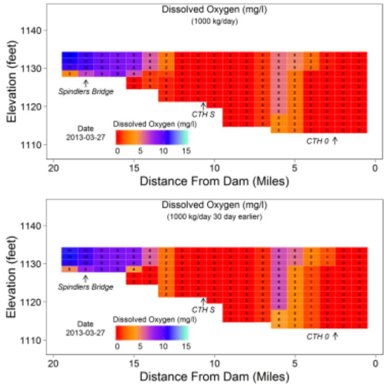
Figure 38. Comparison of dissolved oxygen profiles in the Big Eau Pleine Reservoir for March 27, 2013 comparing earlier start of the aerator and 1000 kg/day addition. Upper profile is simulated 1000 kg/day starting on February 13, second is 1000 kg/day starting 30 days earlier.
