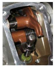
Put Opening shim onto valve stem
