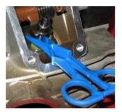
Place a clamp on the valve. In addition to having the cylinder at TDC, this is a little extra insurance to keep the valve from dropping into the cylinder.
