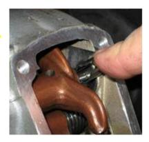
Once the rocker is in place, press the spring clip into place. Some firm pressure will be required.
