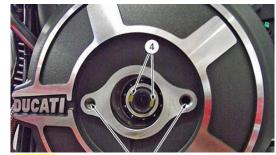
making sure the tangs on the tool engage the indents on the crank shaft (4).
