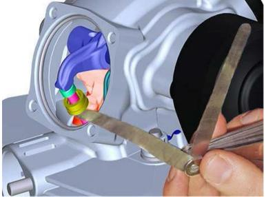
Closing Shim Clearance Once the opening clearances have been measured, measure and record the closing clearances.
