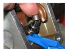
Remove the Opening shim (6) from the valve stem.
