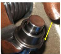
Obtain the correct shim(s) and reassemble the valve train. Slide the closing shim onto the valve stem. The wider side slides onto the valve stem first.
