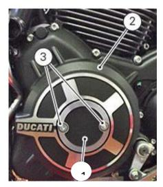
Working from vehicle left-hand side, loosen the two screws (3) and remove plug (1) from generator cover (2)
