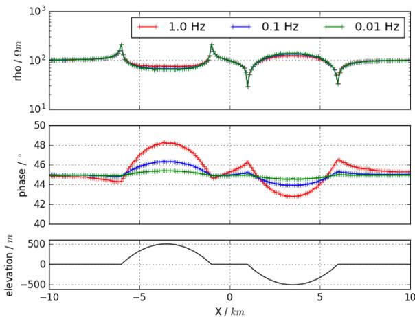
**Figure 3:** The apparent resistivities (top) and phases (middle) for the topography model of XY mode. The figure on bottom shows the elevation of the receivers.
