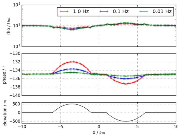
**Figure 4:** The apparent resistivities (top) and phases (middle) for the topography model of YX mode. The figure on bottom shows the elevation of the receivers.
