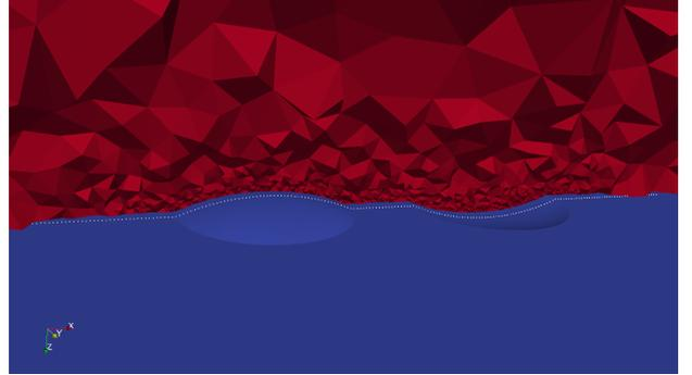
**Figure 2:** The topography model with a spherical hill and valley. The white dots indicate the profile along which apparent resistivity and phase values are computed.
