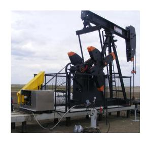
An exciting new solution to powering remote location pump jacks. Utilizing a 27 horse power, oil cooled 2 cylinder engine, the CH740 Power Pack provides a lightweight and easy to maintain alternative to larger, single cylinder engines. Designed to efficiently run on either propane or
