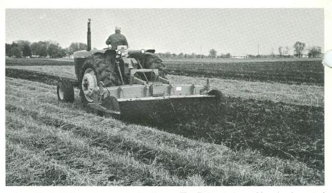
In particularly heavy, compacted soil, the addition of a Howard Rotachisel attachment will dig deep and crack hardened subsoils. The clods are lifted up into the rotor blades and chopped fine, making the field ready for seeding, free of hardpan, and with proper drain-
