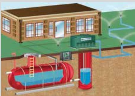
The SkyHarvester product line provides a single-source solution for water harvesting systems at new or existing building sites. Most systems collect rainwater from building rooftops or parking lots for use in landscape irrigation.
