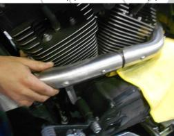
• Slide front "Y" pipe into cross-over pipe and front head port, then attach spring
