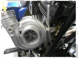
• Loosely attach tail pipe to turbo assembly
