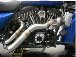
• Line up both tail pipes and tighten hardware
