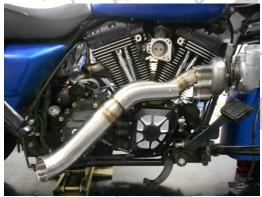
• Loosely mount wastegate to rear tail pipe and waste gate tail pipe to wastegate.
