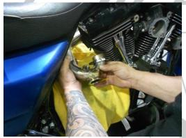
• Slide cross-over pipe into rear head pipe
