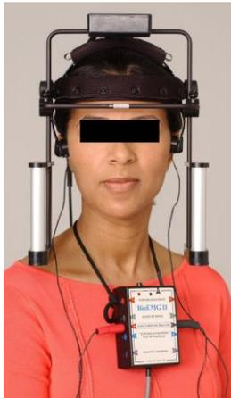
Fig. 4. JT-3D\* Jaw Tracker used together with EMG to monitor a bite registration
