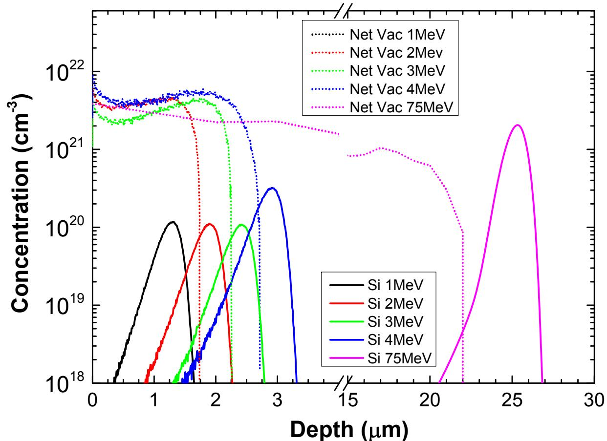
Increasing implant energy allows depth of V-rich region to be extended
