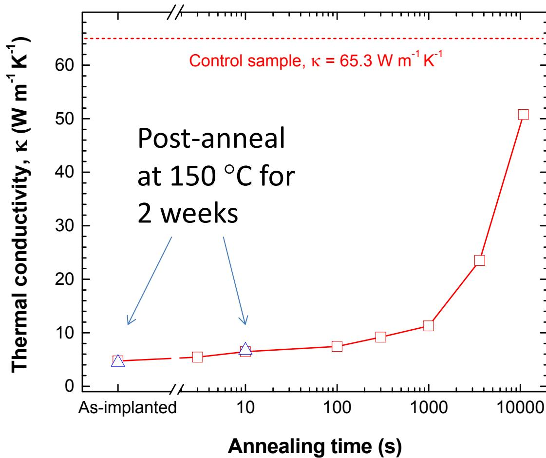
TEGs must be exposed to high temp in order to work!
