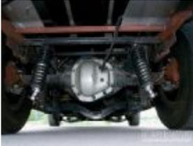
The custom Dana 60 rear axle, four-link, coilover shocks, and crossmember were all built by Joe.
