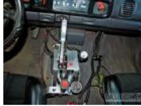
A custom raised shifter pedestal was made to put the shifter within easy reach.
