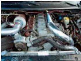
The intake manifold, compound turbochargers, nitrous setup, exhaust manifold, and intercooler all had to be custom made.
