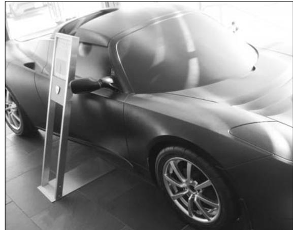
Inside were a couple of non-functional but historic Teslas: The flat-black Aero Buck, (*above*) which was computer-machined from solid fiberboard from the scans of the original clay model, and used for wind tunnel testing, and the hand-built “Drivetrain Mule,” the second engineering vehicle built by the company and the first to resemble the Roadster’s final design.
