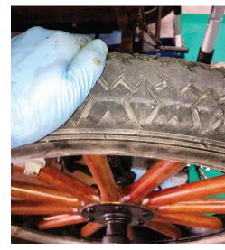
In the photos above, the wheel felt solid on the spindle, but with the wood wedge removed there was perceivable rocking, indicating the spindle body had some wiggle.
