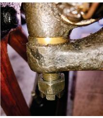
Finally, hold the upper head of the spindle bolt that has been adjusted, in place, with one wrench. At the same time, tighten the castle lock nut firmly with another wrench and align the cotter hole. Replace that safety cotter pin to secure and lock the nut.
