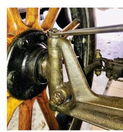
Clear the cotter pin hole and replace the castle lock nut, as shown in the photos below.
