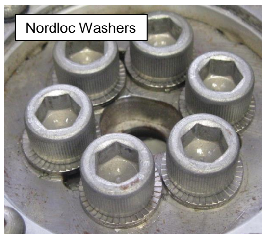
Figure 10 – Flywheel fitted with Nordloc washers
