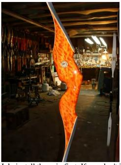
I do install the coin first. If you don't install it before spraying and get any finish in the hole it will build up and can even make the wood swell a little and the coin will not fit. On the raised plastic buttons I install those after all the finish is on. Some finishes will react funny on plastic.
