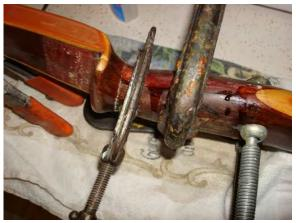
Add 2-3 more clamps wherever you can, Good idea to stay as near the crack as possible.5 clamps with about 2-3 pounds of pressure each. Now wait about 12-24 hours until the LT gets inside the crack which is not getting exposed to the air so much will have plenty of time to dry
