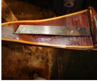
Once you have either used a small scraper or sand paper and removed all the dry glue. Most of the old finish will get scraped or sanded off as well. Check and see if the gap is filled. If not get a pick or small nail and remove all the uncured glue. Then fill it again.
