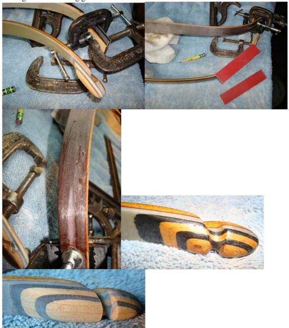
Hey Shawn if the color is not coming back to good. You can use a small scraper and shave off like 1 MM of the wood with no problem's that really helps bring the color back. Then let the bow set at room temp or up around 80-90 degrees even for 3-5 days that brings the natural wood color back.
