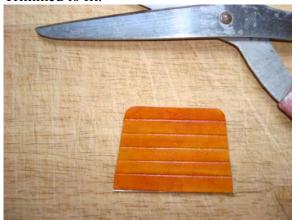
Remove protective backing from tape.
