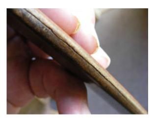
Here are a few more pics of tip overlay repair for Shawn. The 60" 1957 Kodiak Special has factory wood & paper tip overlays. I had to replace one and used wood & black fiberglass to make the repair. The red canvas micarta in the pic will be to make underlays for the 66" KS. It has a tiny bit of fiberglass damage on the belly side right near the string grooves.
