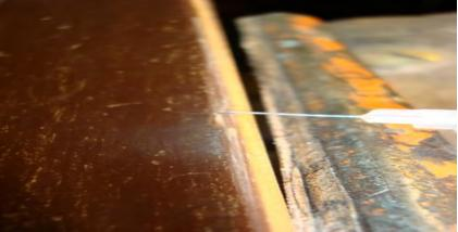
See those? Bear Archery would tell you to break those off with a pair of needle nose pliers so they do not snag on anything and paint over that spot with some clear finger nail polish. I like to glue them down and wait 24 hours and then pick at them with the needle of the syringe. If any are not glued down, I normally try and sand them out when ever possible.
