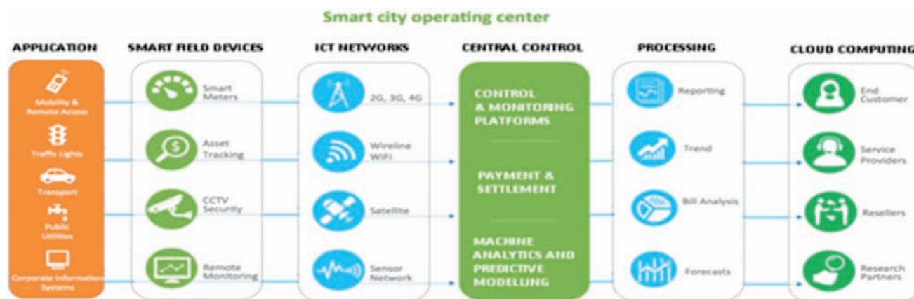
Figure 2. Smart City Operating Centre
