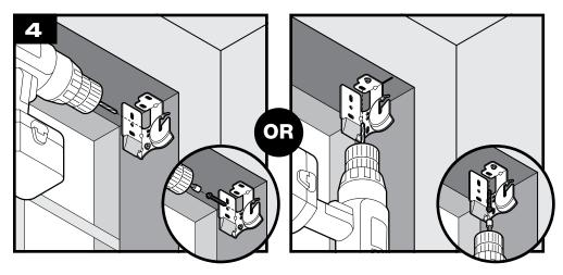
**SIDE MOUNT:** Drill second 3/32" pilot hole. If necessary, use wall anchor (not included). Secure brackets with second screw using a 1/4" driver. **TOP MOUNT:** Drill second 3/32" pilot hole. If necessary, use wall anchor (not included). Secure brackets with second screw using a 1/4" driver.
