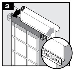
Dry fit top shade and check vertical side gaps and if shade is level. Adjust brackets if necessary by loosening screw and moving bracket down in slot. Once level, remove shade and tighten screw.
