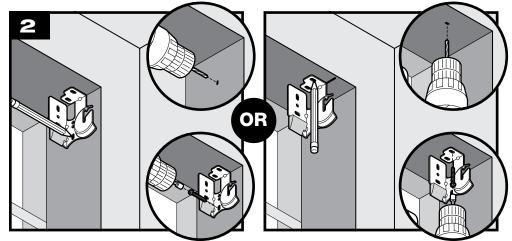
**SIDE MOUNT:** Mark bottom of slotted hole on side of bracket. Drill 3/32" pilot hole on mark. If necessary, use wall anchor (not included). Secure brackets with one screw using a 1/4" driver. **TOP MOUNT:** Mark center of slotted front hole on top of bracket. Drill 3/32" pilot hole on mark. If necessary, use wall anchor (not included). Secure brackets with one screw using a 1/4" driver.
