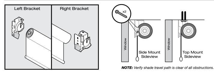
**NOTE:** Before you begin, verify shade will fit opening. Adjust depth to establish proper clearance for shade in full open position and so that full up position is not in front of opening.
