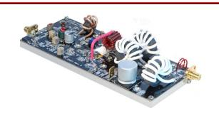
The RFP27.12-150XR is a high gain Class A/AB XR-rated amplifier designed specifically for the 27.12MHz ISM band. It is ideal as a driver stage or output PA in high power industrial, commercial, or scientific systems. Its XR rating ensures ruggedness when driving mismatched loads such as plasmas. It is supplied with SMA input and output connectors.
