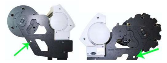
3. Next, attach the Fabric Catch Arms to the inside of your Fusion Revolver or Racket with the ¼" x 20 Button Head Screws and Locking nuts provided in your fabric catch
