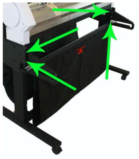
4. Finally insert the last two poles into the last two slots on the fabric catch. The catch arms allow you to slide the front facing pole to a closed or open position. Rest the poles in
