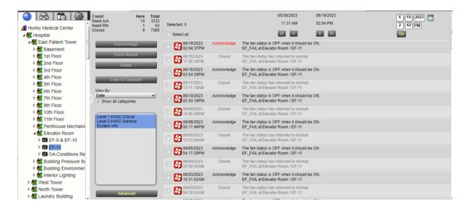
Alarms are being issued and recorded that appear to be in error and are non-sychronous to operation of the unit EF-11.
