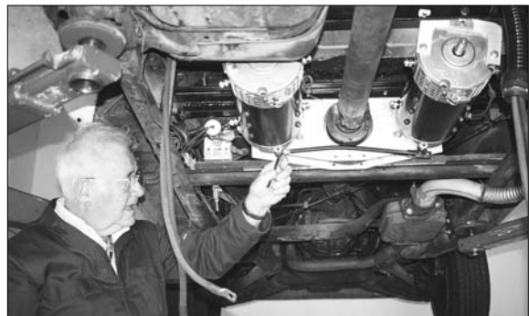
Paul putting finishing touches on the two offsetting Advanced DC electric motors which are coupled to the mid point of the drive shaft of the rear wheel drive S-10 pickup. The motors are connected to a cogged pulley on the drive shaft by a serpentine belt. The pulley has a one way clutch which allows the gasoline motor to drive the shaft when the electric motors are not in use.
