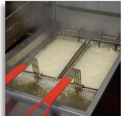
Heated cooking oils can create an ignitable vapor:air mixture in the commercial kitchen.
