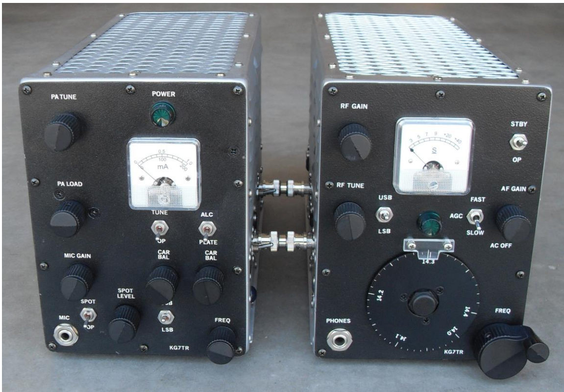
Figure 1: The Vintage SSB Special Radio Set connected for transceive operation. This picture shows the latest configuration. The transmitter meter switch now has an ALC position in place of the previous GRID position, and the receiver has a new S meter.
