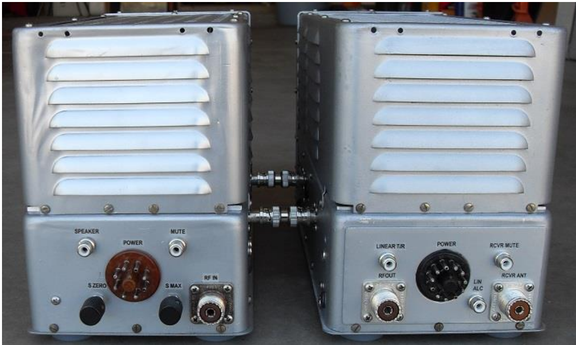
Figure 2: Rear view of the set showing the new SO-239 RF connectors and the RCA jacks for linear ALC, linear T/R and receiver mute.
